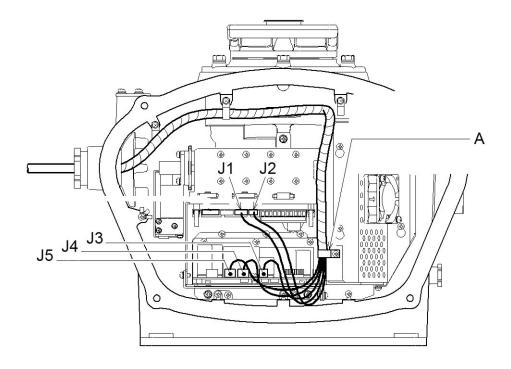
7. Connect the five interconnection cable connectors (B, C, D, E, and F) to the J connectors as follows:
